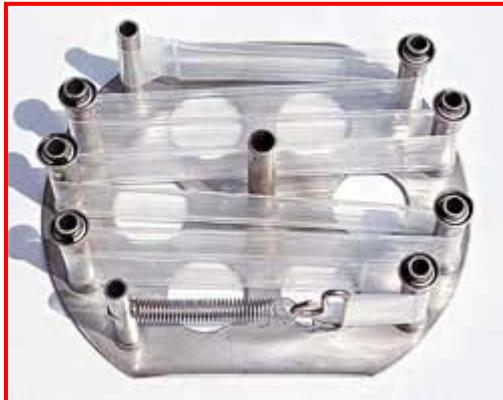
Figure 1. Spider carrier with mounted lipid filled membrane for SPMD sampling.
