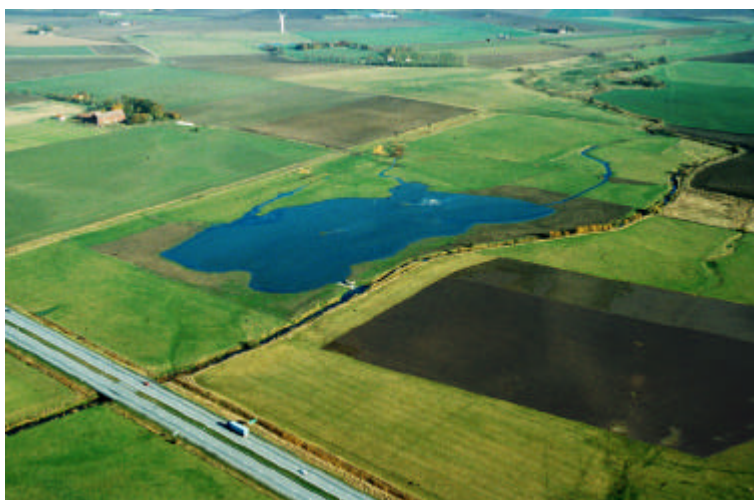
Figure 14. The wetland in the picture has a size of 6 hectares and is the largest in the project. Because the main stream is very deep, with a water level far below the ground level, the water had to be fetched 850 meters upstream. The water runs first in a culvert and in the end in an open channel.
