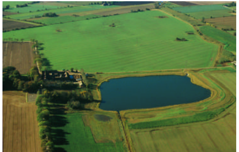
Figure 13. In irrigation ponds environmental benefits are combined with a commercial benefit for the landowner. In this irrigation pond with a size of 5 hectares, more than 100 000 m 3 water is stored during the winter season for irrigation purposes during summertime.
