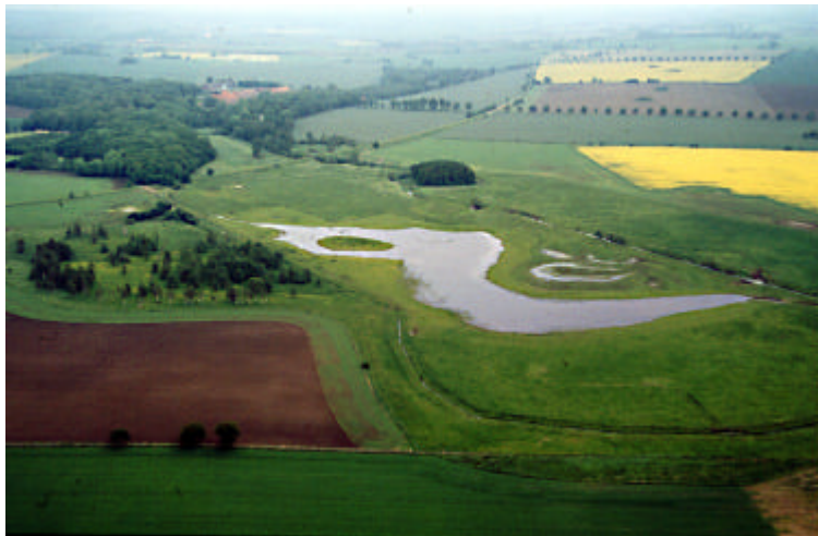
Figure 12. A shallow water with a size of 5 hectares has been constructed in the watershed of Kävlinge river. The inlet from a main contributory stream is located 600 meters upstream and the water flows to the wetland in a long channel.
